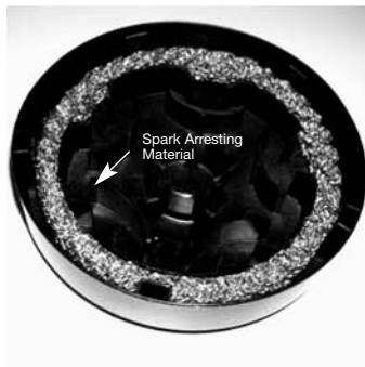
check for spark arresting material
